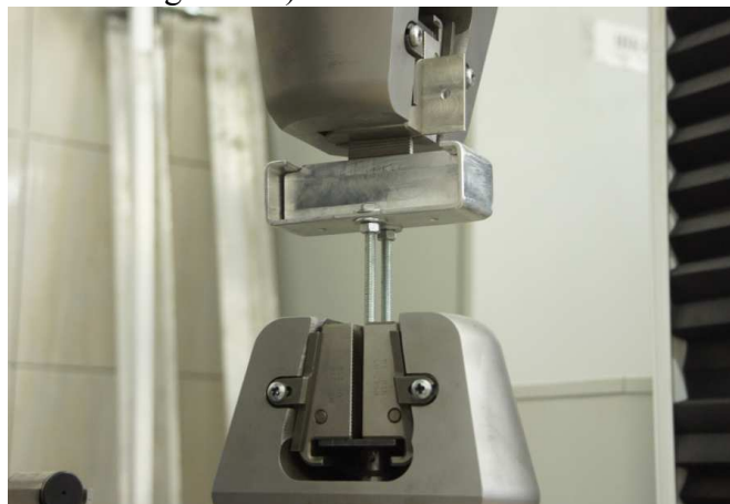
Figure 5. General view of tester with subframe specimen
