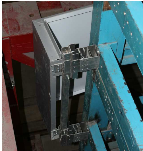
Figure 6. General view of mounted façade cladding element (side view)
